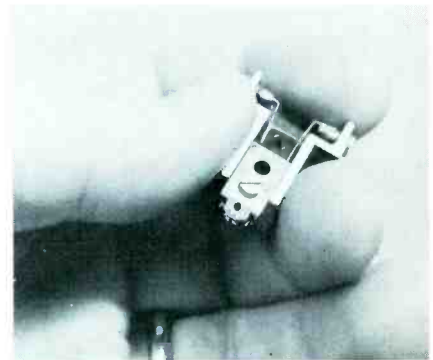
Fig. 13 Each tiny video head is fastened to a plate assembly, which has provisions for electrical continuity, and for precise mechanical adjustments.
