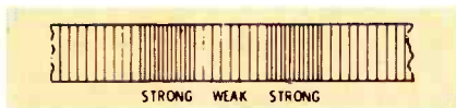
Fig. 1 Varying current through the recording head magnetizes the particles of iron oxide, leaving areas of strong and weak magnetization that can be "read" during playback.
