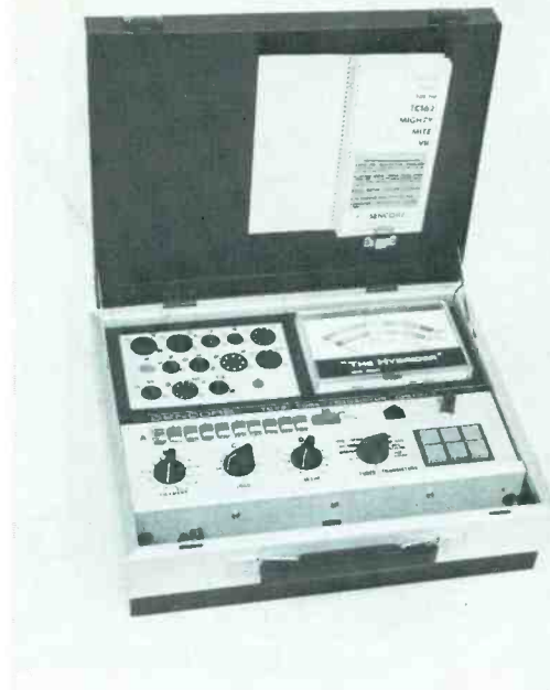
Fig. 1 The Sencore Model TC28 tests both tubes and transistors, with all test readings shown on the meter. In addition, an audio tone (Cricket) sounds when a transistor has gain. It's not necessary to connect the transistor leads in any certain way. A tube-testing booklet and simplified instructions for both tube and transistor testing are printed inside the lid. This instrument is an improved combination of the Sencore Mighty Mite VII tube tester and the Cricket transistor tester.
