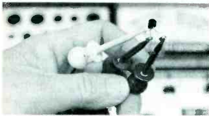
Fig. 6 Three EZ Hook clips securely grasp the transistor leads. To use a clip, slide back the sheath to expose the curved hook, insert the wire, then release the sheath, which by spring pressure holds the wire in the hook.
