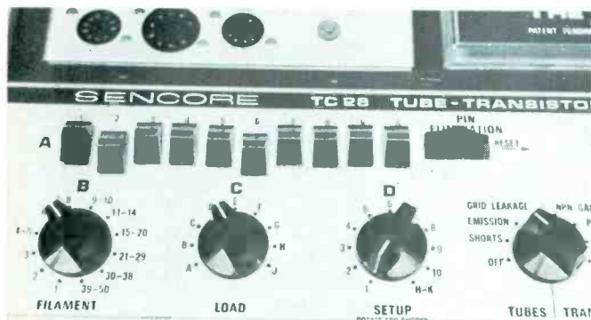
Fig. 3 Ten pin-elimination switches open the circuit to any duplicate pins to prevent false short indications. The "B" switch sets the heater voltage, "C" switch determines the applied voltage and the load resistance, "D" switch is set for the grid (or rotated to all positions for shorts test), and the "Tubes/Transistors" switch selects the specific tube or transistor test.
